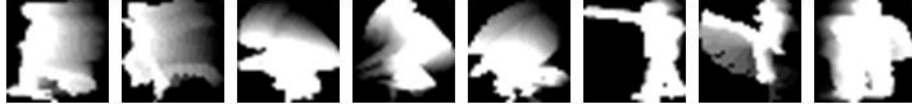
Fig. 8. Sample normalized MHIs (from the left: walking, running, sitting, standing, falling, punching, kicking, and turning) for the training of a multi-layer perceptron.
